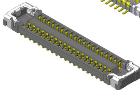
The WP27D Series is a 0.35mm pitch low-profile stacking type board-to-board (FPC) connector with special hold-downs that can be used as power supply terminals, and is ideal for high-density mounting in slim and compact information communication devices like smartphones. This product has a structure that adds protection to the mating surface to prevent damage to the insulator in case force is applied while connectors are misaligned. Also the hold-downs can be used as high-current terminals.
