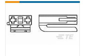
TE Part #623346-1 2P CONNECTOR HOUSING
