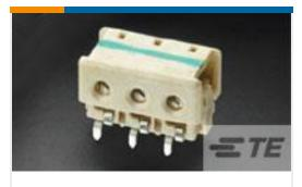
TE Part #2106751-4 Connector, Thru Hole-IDC, 4 pos, 18AWG
