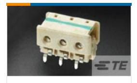
TE Part #2-2106751-4 Connector, Thru Hole-IDC, 4 pos, 22AWG
