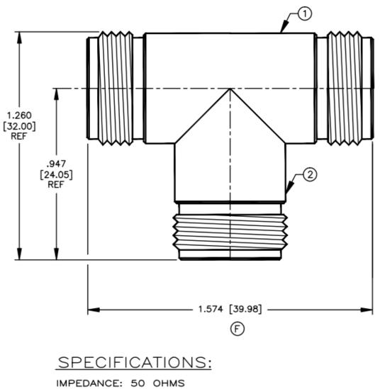
WORKING VOLTAGE: 1000 VRMS @ SEA LEVEL FREQUENCY RANGE: 0-11 GHz INTERFACE PER MIL-STD-348A, SECTION 304.2
