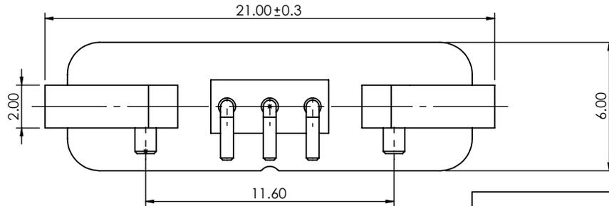
MAGNETIC SPRING LOADED CONNECTOR,
