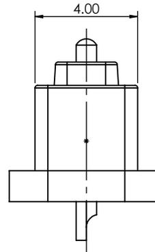
MAGNETIC SPRING LOADED CONNECTOR,
