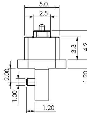
MAGNETIC SPRING LOADED CONNECTOR,
