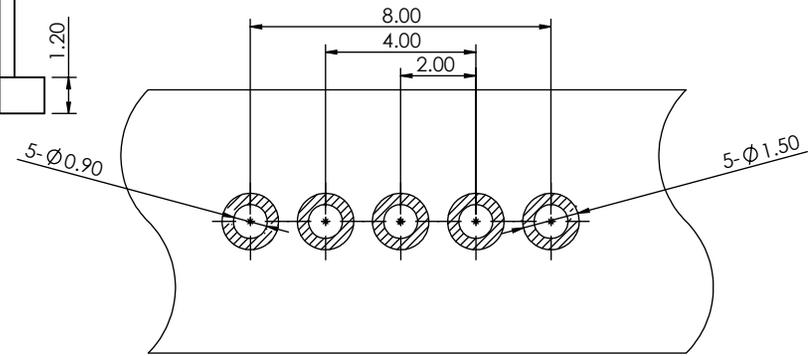
RECOMMENDED PCB LAYOUT (T:1.6mm)
