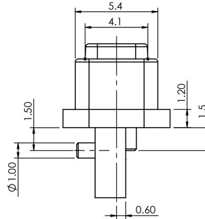
MAGNETIC SPRING LOADED CONNECTOR,
