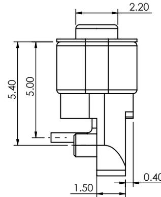
**MAGNETIC SPRING LOADED CONNECTOR,
