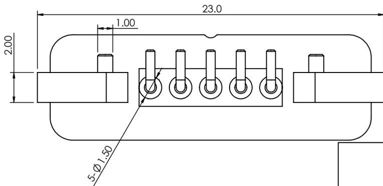
MAGNETIC SPRING LOADED CONNECTOR,
