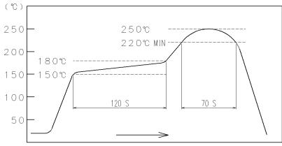
FIG – 1 <u>RESISTANCE TO SOLDERING HEAT</u> (TEMPERATURE AT TOP SURFACE OF CONNECTOR)
